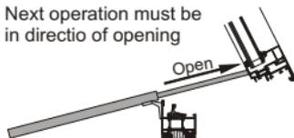
**The actuator will be destroyed when multiple triggering in end position "Open" or "Close" happens!**
